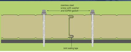
Hipertec® Wall is a sandwich panel with non-combustible insulation core made of rock wool and suits best to meet today's high requirements for fire protection and sound insulation. Depending on the core thickness the fire resistance may reach up to 120 minutes. High support widths and an easy installation both vertical and horizontal-make this product very cost effective, perfectly apt for application as
